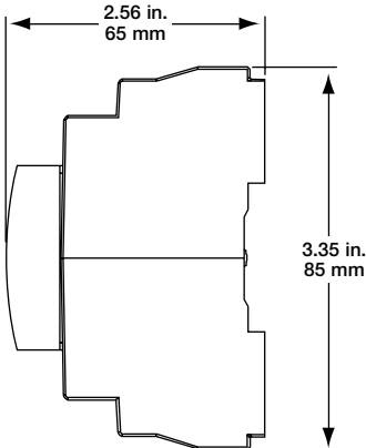
View of the Ethernet Network Interface showing height and depth
