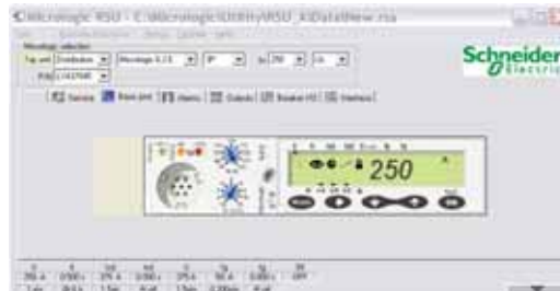
RSU mini-supervision screen for current measurements.
