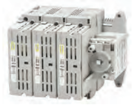
Compact Fused Disconnect Switch accepts Class "J" fuses. Fuse holders are top mounted for easy access. The switch accepts auxiliary contacts for control circuit applications including the ON/OFF control of remote pilot lights or signal for programmable controllers.
