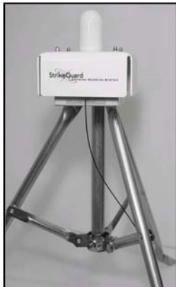
Lightning Warning System
