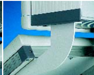
Enclosure bar connector Tilting angle 120°, rigid, for enclosure installation depth 44 mm (1.73")
