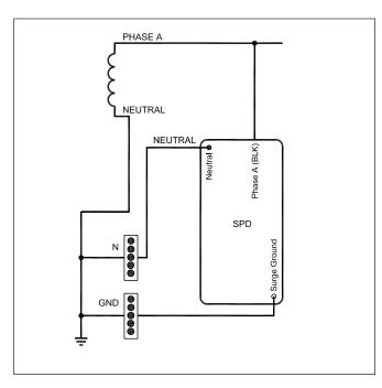
Figure 12. Wiring - Single Phase Units (230 L)
