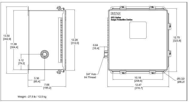
Figure 6. NEMA 4-4X (With Disconnect) (Suffix O, Q))
