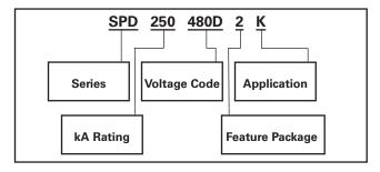
For example, a 480 volt Delta (3-wire plus Ground) for use in an NEMA 1 application requires an SPD model SPD 250480D2K, where:
