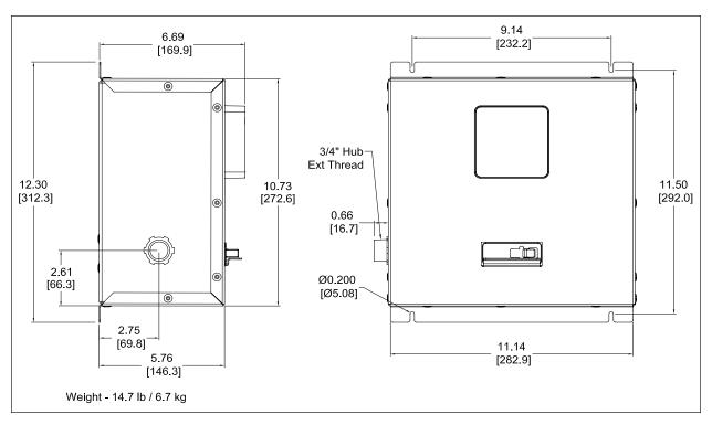
Figure 5. NEMA 1 (With Disconnect) (Suffix M)
