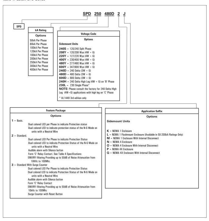
Example: SPD 250480D2K = SPD Series, 250kA Per Phase, 480D Voltage, Standard Feature Package, NEMA 1 Sidemount Application.
