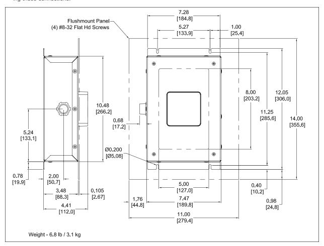
Figure 2. NEMA 1 (With Flushmount) (Suffix L)
