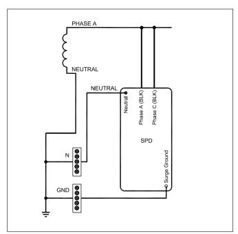
Figure 13. Wiring - Single Phase Units (240S) for 120V Single Phase Applications
