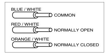
Figure 7. Sidemount Form C Wires
