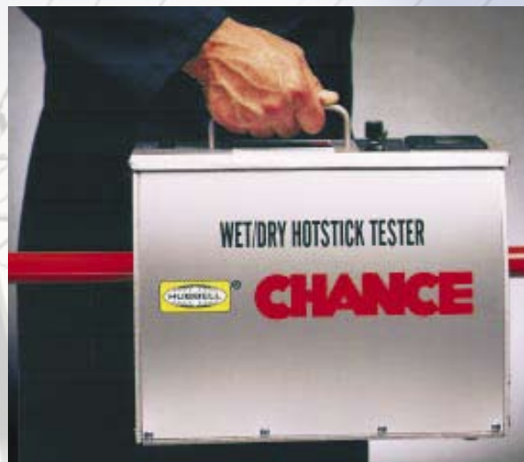
For wet or dry testing, unit simply takes overlapping readings along the full length of any hot stick up to 3-inch-diameter.
