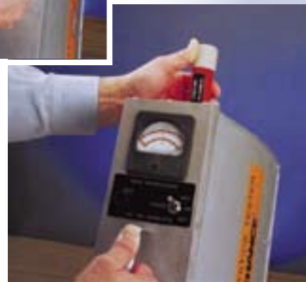
Before each use, set the meter needle to zero with nothing in the Tester and self-test the Tester with the Check Bar included.
