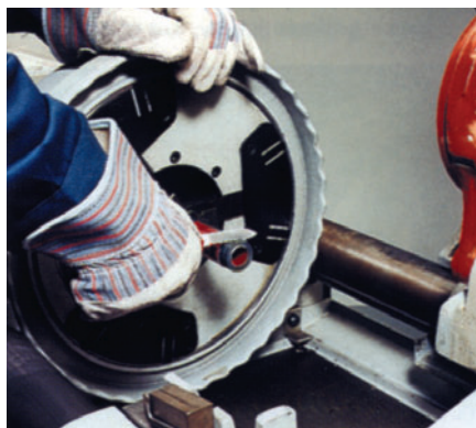
The PVC coating may need to be pencil cut in order that the die teeth may engage the conduit.
