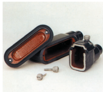
The V Seal™ gasket system on form 8 condulets sizes 1/2" through 2" effectively seals the fitting with a male female interlocking groove.
