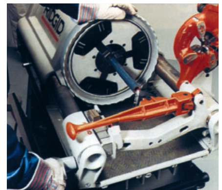
Use a reamer to remove rough edges.
