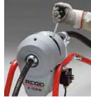
Release handle, cable stops instantly.
