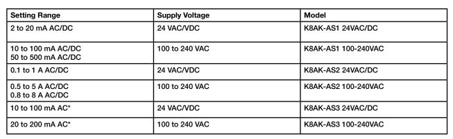
\*K8AK-AS3 is designed to be used in combination with OMRON K8AC-CT200L Current Transformer (CT). (Direct input is not possible)
