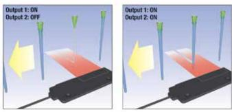
In combination with the twin output function of the E3X-DA-S amplifier, the diffuse reflective area monitoring fibers can detect very small objects (e.g. needles) and a second state (e.g. cover present). The area beam compensates for position variations at high speed.
