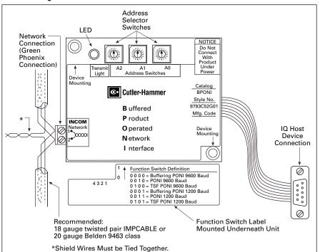
BPONIs and IPONIs may be daisychained together with other IMPACC devices on a common twisted shielded pair network.
