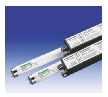
SYLVANIA OCTRON EXtended Performance Super ECOLOGIC® lamps and dedicated QUICKTRONIC® programmed start electronic ballasts form a lighting system that provides up to 22% energy savings and comparable light output with twice the lamp life of standard instant start T8 systems. The "soft" start of the programmed start ballasts makes this system the choice for frequent switching cycle applications.
