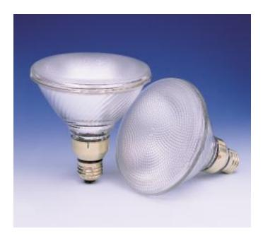
SYLVANIA METALARC POWERBALL CERAMIC lamps meet today's color-critical needs by combining conventional metal halide pulse start characteristics, such as good efficacy and long life, with improved lamp-to-lamp color consistency and high CRI. SYLVANIA's POWERBALL lamps use a patented rounded arc tube shape, which allows for more uniform temperature and improved color consistency.
