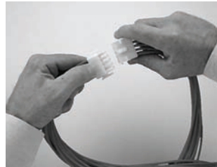
Logic Disconnect Plugs
