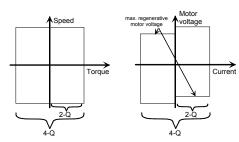
Regenerative (4-Q) power converter modules are used when motor torque can occur in either direction. This is for applications such as:
