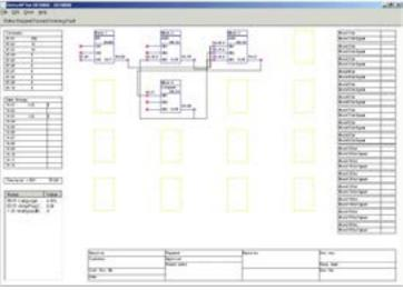
One page is freely configurable by the user. An individual commissioning sequence or parameter selection can be setup to application, machine or motor demands.
