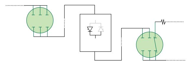
Either an AC or DC contactor is required, but not both.
