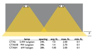
Meets Life Safety Code standard minimum illuminance of 0.1 FC and average illuminance of 1.0 FC. Assumes open space with no obstructions, mounting height: 8', ceiling height: 9', and reflectances: 80/50/20. Analysis based on independently tested photometrics.
