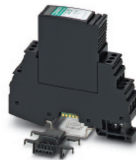
2-wire with common reference potential, 9/10 connection grounded via gas-filled surge arrester
