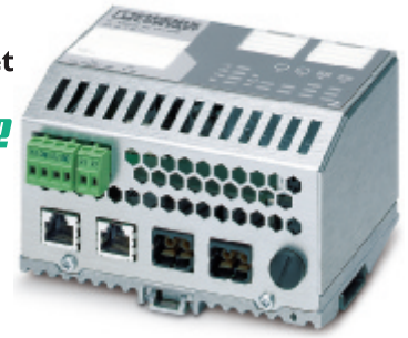
2 RJ45 ports and 2 POF SCRJ ports
