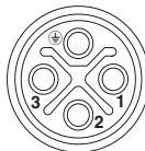
Connector pin assignment of M12 socket, 4-pos., S-encoded, view of socket side
