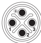
Connector pin assignment of M12 plug, 4-pos., S-encoded, view of pin side
