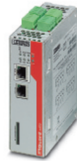
Router with intelligent firewall
