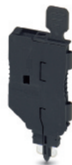
5.2 mm fuse plug, for 5 x 20 mm cartridge fuses
