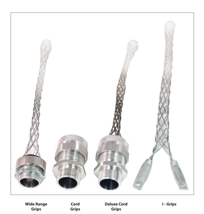
Ericson's Strain Relief Grip and Mesh eliminates cable pullout to reduce a loss of service resulting in costly downtime. The endless mesh weave provides easy cable installation that is woven with stainless steel providing corrosion resistance for all applications. A NPT and PG threaded body allows for easy attachment to either a threaded hub or knock-out in box.
