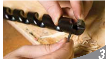
Tighten Set Screw.
