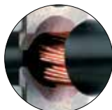
Round stripping blades on Pro 16 cut insulation cleanly
