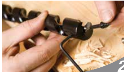
Insert Feed Screw...
