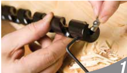
Insert Cutting Edge...
