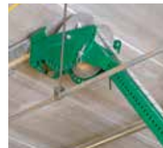
Optional 12' boom extension for high pulls
