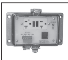
Network Tap PC Board with 120 VAC Duplex GFCI with internal Simplex GFCI & 3 Amp circuit breaker
