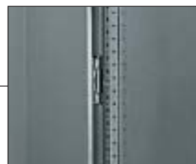
Stainless steel inside guide and reinforcement frame with section 18×18 mm, reinforced at 25 mm intervals with Ø 5 and 10 mm drill holes.
