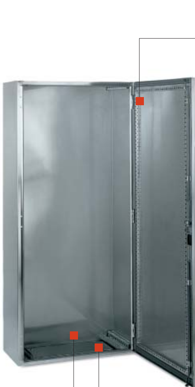
Stainless steel inside guide and reinforcement frame with section 18×18 mm, reinforced at 25 mm intervals with Ø 5 and 10 mm drill holes.
