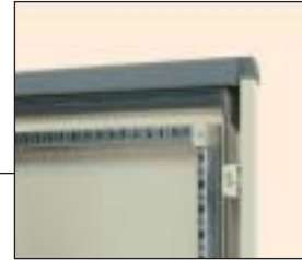
Inside view of the 2 mm thick door with detail of 15 × 20 mm cross section reinforcement frame with Ø 5 and 10 mm drilling every 25 mm.
