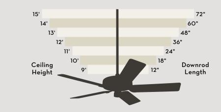
Note: For best performance and appearance, an extension downrod should be used with your Casablanca fan when installing on a high or sloped ceiling. Casablanca offers extension downrods in lengths up to 8' (96"). The chart lists the most common ceiling heights and suggested downrod lengths. For safety reasons, the fan blades must be a minimum of 7 feet above the floor. For more information, see your Casablanca dealer.
