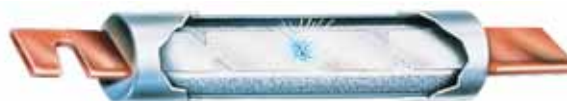
Figure 2. Under sustained overload, a section of the link melts and an arc is established.
