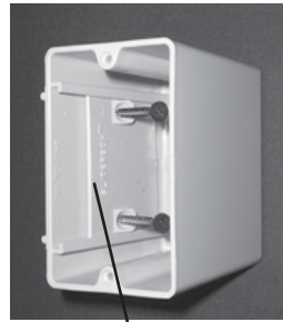
Slider plate retracted sets box in fully adjusted forward position for maximum wall substrate thickness of 1 3/8".
