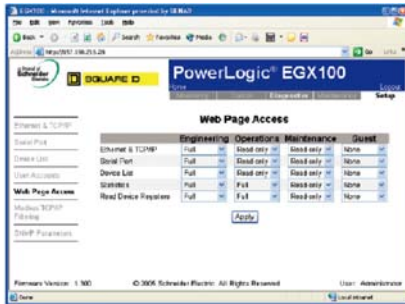
EGX100 lets the Administrator assign access to setup pages by user groups
