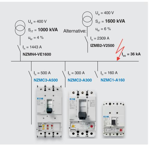
Circuit-breakers from the new C series with 36 kA short-circuit breaking capacity and nominal current from 20 - 500 A are the correct choice for the most frequently used standard applications. The decisive factor for the level of the short-circuit current in the most widely used low-voltage radial networks is the capacity of the low-voltage transformer.
