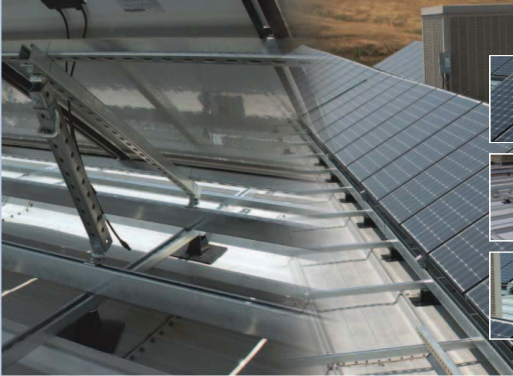
P1000T Attach to P1000HS with 1/2" JHCS & P3010 Stout Nut & Thru the Half Slot in the P1000T with 1/2" JHCS. HPLW037
