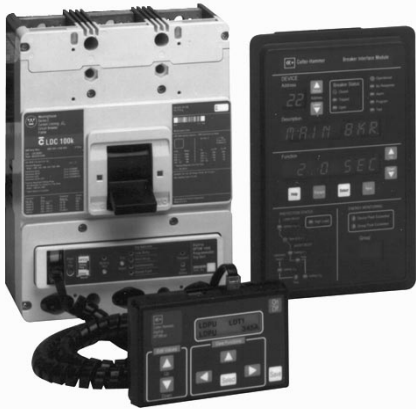
Digitrip OPTIM Trip Units can be programmed with hand-held OPTIMizer (above) that plugs into the front of the trip unit; or with the Breaker Interface Module mounted directly on the enclosure door.
