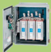
The SG320 Series is a modular hardwired suppression device and recommended for all ANSI/IEEE Category locations. Contains one bolt-on module per phase for easy maintenance.
