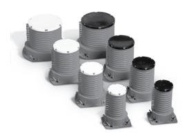
These firestop devices are designed to make firestopping through concrete easy and affordable. With models available to accommodate plastic or metallic pipe, 3M<sup>™</sup> Fire Barrier Cast-In Devices are installed prior to the concrete pour (attaching directly to the wood forms) and can be adjusted to various concrete depths.
