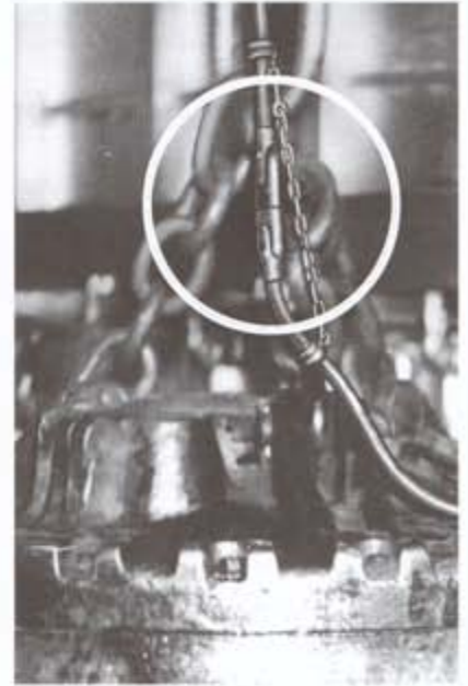
Weather-tight, dust tight, plugs with strain relief chains allow easy removal and replacement of electro-magnets.
