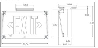
Mounting: wall mount, ceiling mount, end mount Conduit Entry: top, bottom, or either side of the unit
