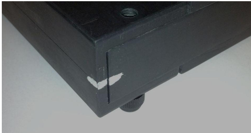
Figure 7: Hash Marks on Split Core CT
