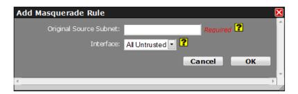
**Original Source Subnet:** Enter the subnet, using IP/CIDR notation that will be masqueraded out a specific interface. All traffic that is sourced from this subnet and that is destined to go out the specified interface, will be masqueraded with the source IP address of the interface specified. (Required)
