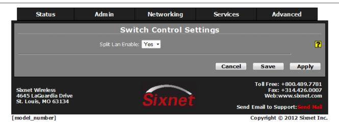
This mode is only available on RAM-6x21 - 5 port equipped hardware. The purpose of the Switch Control function is to create a WAN/LAN separation similar to what is seen on the R series router. This gives the user the ability to create a divided network with additional capabilities.
