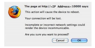
• Click on the "OK" button the reboot the Sixnet router remotely.
