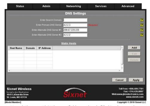
The Primary, Alternate #1, and Alternate #2 DNS server fields are already filled in; they are the current servers in use by the Sixnet router.
