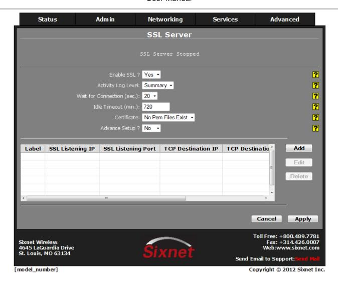
**Activity Log Level:** This controls the logging level for SSL Connection activity. Recommended setting is "Summary" for a production, and "Full" for test environment.
