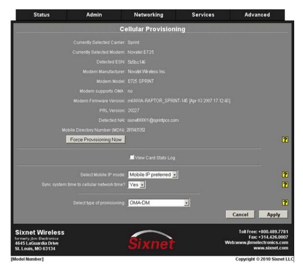
Simply select OMA in the dropdown option and click apply. This will already be the default operation of OMA capable devices. When a connection is refused by the tower, the unit will automatically attempt automatic provisioning at regular intervals. You may click "Force Provisioning" to cause an immediate OMA attempt.
