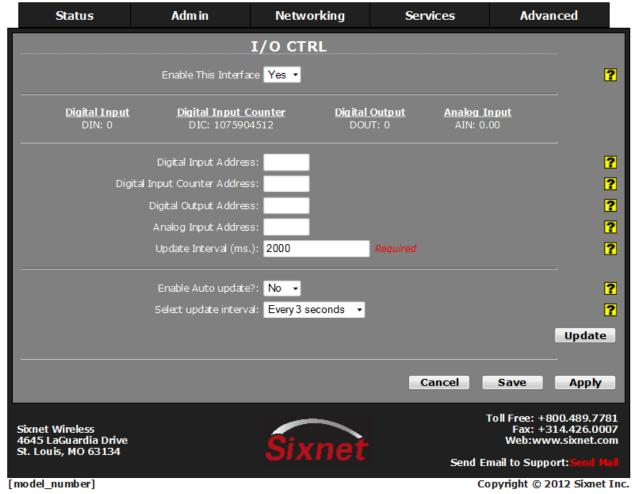
Digital Input Address: Enter the address of internal IODB database for Digital Input I/O control. Valid Values: 1 through 65535 as defined for specified I/O type.
