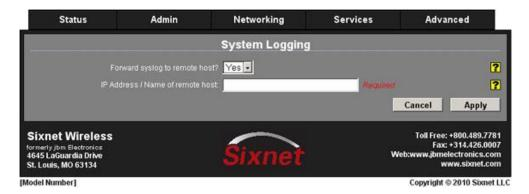
**IP Address / Name of remote host:** Enter the IP address of the remote syslog server to which you want to forward messages.
