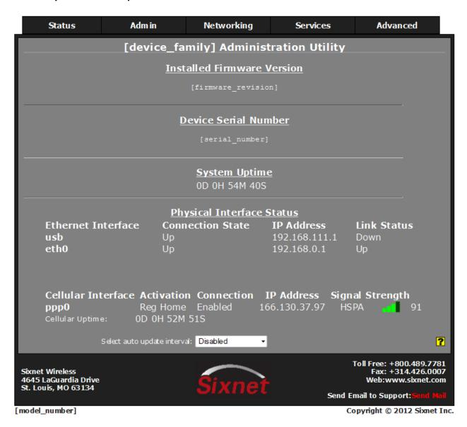
At this point, you are connected to the Sixnet router and can configure it to meet your needs.
