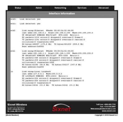
The "Details" menu item will display a more system specific description of the interfaces on the Sixnet router.
