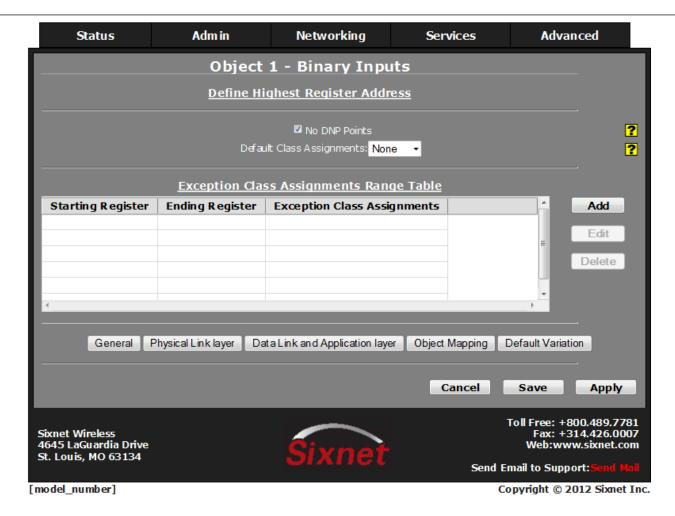
Important Note: Each type of I/O must have its corresponding Object Mapping Window opened at least once, or else the I/O won't be mapped.
