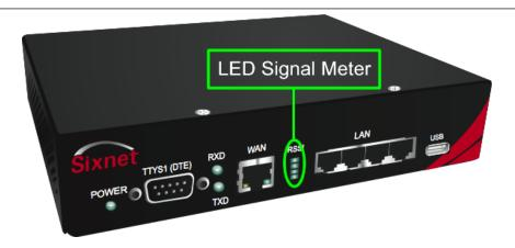
If the top and bottom LEDs are flashing, the device is not receiving sufficient signal from the cellular towers in order to be able to connect to the network. Typically, 2-3 LEDs of reception are a minimum requirement for a sustainable connection. If it is displaying bars of signal that flash every 2 seconds, then signal is available to the tower, but a cellular connection has not been established.
