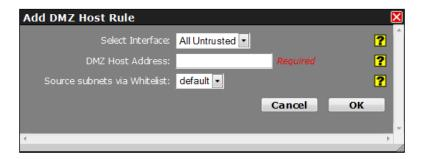
**Select Interface:** Click on the pull down menu to choose an interface that will be forwarded to a DMZ Host. All incoming packets (TCP/UDP/ICMP/etc) will be forwarded to the DMZ Host specified.
