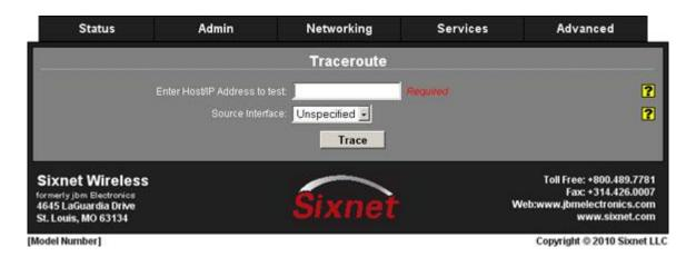
Type in the IP Address or URL you wish to trace and click on the "Trace" button to use any interface that the router determines as having the route to the designated address.
