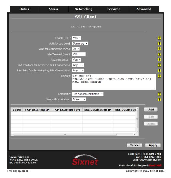
**Bind Interface for accepting TCP Connections:** This will restrict the unencrypted listening socket to allow connections coming into the specified interface only. Recommended setting is "Any".
