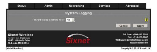
• Click on the pull down menu for "Forward syslog to remote host?" and choose "Yes" to reveal the system logging configuration fields
