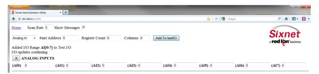
The messages log shows that we have "Added I/O Range AI[0:7] to Test I/O" and now we see each register that can be edited and monitored for the Analog inputs.
