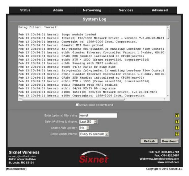
You have the option of selecting the number of lines to display, enable the auto update function and set the frequency of the updates interval.
