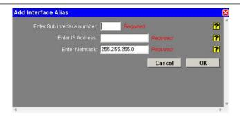
**Enter Sub interface number:** Enter the desired Sub interface number in the file provided. The valid range is 0-99, and each aliased interface must be uniquely numbered. The final sub interface name will then be in the form **ethx:y** where **x** is the root interface number and **y** is the sub-interface number.
