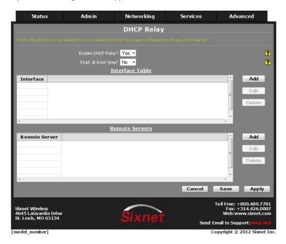
DHCP Relay will enable a service that will allow you to connect a local interface with a remote DHCP Server.
