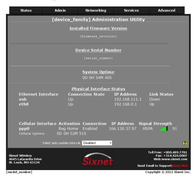
As shown, the router is receiving good signal from the cellular network, it is connected, and has been issued an IP address.
