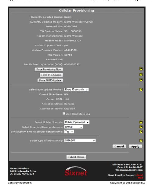
Select which type of Provisioning you will be using. There are six (6) different types of provisioning:
