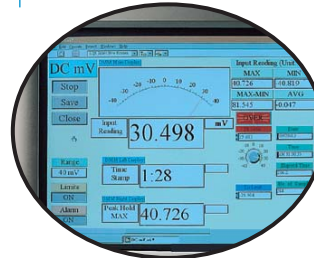
Data acquisition and analysis with 490 ProVision™ software.
