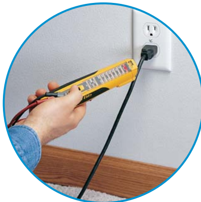
Non-contact voltage sensor easily locates breaks in power cords.
