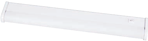
P7021-30EBWB White One, 13wt T5 Linkable Size: 3-1/4" W., 1-1/8" ht. 21" L. Lamp: One F13T5 lamp, 13w max. (included).
