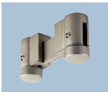
P8778-09 Brushed Nickel Illuma-Flex Power link. Electrically links two sections of track together. Designed to be used with or without support stem. Size: 3-3/8" W., 1-5/8" ht.
