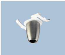
P8781-09 Brushed Nickel Illuma-Flex T-bar Adapter Allows support to be mounted to a t-bar ceiling. Set of six adapters included. Support stems not included. Size: 1-1/2" W., 1-3/8" ht.
