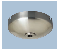
P8780-09 Brushed Nickel Quick-connect monopoint. Includes integral 50w electronic low voltage transformer. Monopoint mounts to an electrical ceiling box. Illuma-Flex fixtures using the P8777 converting adapter (included with all Illuma-Flex fixtures) easily connect to the monopoint with a quick push and turn connection, no fixture to box wiring required. Size: 5-7/8" dia., 3-3/8" ht.
