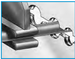
Gripper pads hold the wire securely in a centerline relationship with the blade.
