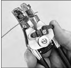
Short stop-latch protects wire strands by limiting the stripping stroke to 5/32 in. and retains the slug until the wire is ready for terminating.
