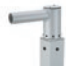
PT-*H Round External Mount Horizontal Tenons (Aluminum) - Mounts to 2.375"-3" (60-76mm) O.D. round aluminum or steel poles or tenons; Mounts to square pole with PB-1A* tenon
