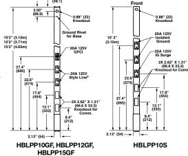
10'2" (3.10m) 12'2" (3.71m) 15'2" (4.62m) 2X 2.62" X 1.31" (66.6 X 33.3) Knockout for Comm 22.6° (574) Mounting Foot with Foam Pad HBLPPO, HBLPPO12, HBLPPO15
