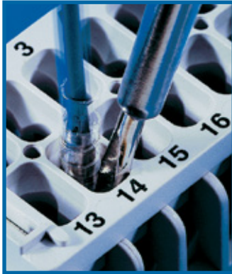
Use small blade screwdriver to push wire entry tab in for easy contact removal.
