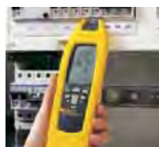
Location of fuses/breakers and assignment to circuits
