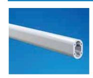
**Support section CP-L**Attachment to the connection components with 4 self-tapping screws in a screw channel, may be cut to any required length, no threadtapping required.
