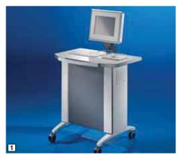
Compact enclosure, ready to connect. Standard commercially available tower PC's, up to 21 x 10 x 24" (530 x 250 x 600 mm) H x W x D (max. 44 lb [20 kg]) may be attached securely to the base, screw fastened to the door using the retaining strap (supplied loose). The rear interfaces of the PC are readily accessible with the door open. Because the socket strip and fan-and-filter unit are already pre-installed, the enclosure is ready for immediate use.
