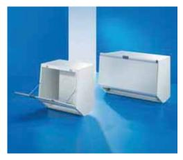
Console for mounting on pedestal with depth 20" (500 mm) in conjunction with desk unit. Opening at the rear, with rear panel hinged at the bottom and cam locks. Side panels with bolts for mounting rails for interior installation.
