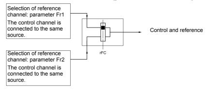
Parameter rFC can be used to select channel Fr1 or Fr2 or to configure a logic input or a control word bit for remote switching of either. See the detailed diagrams on pages 30 et 32.
