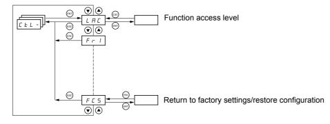
The parameters can only be modified when the drive is stopped and no run command is present. On the optional remote terminal, this menu can be accessed with the switch in the  $\cap$  position.
