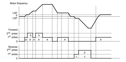
This type of +/- speed is incompatible with 3-wire control.
