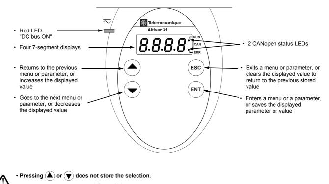
• Press and hold down (>2 s) (lacksquare ) or (lacksquare) to scroll through the data quickly.
