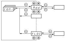
The parameters can only be modified when the drive is stopped and no run command is present. Modifications to parameters Add, tbr, tFO, AdCO and bdCO are only taken into account following a restart. On the optional remote terminal, this menu can be accessed with the switch in the  $\Box$  position.
