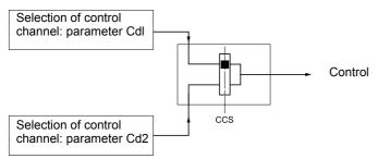
Parameter CCS can be used to select channel Cd1 or Cd2 or to configure a logic input or a control word bit for remote switching of either.
