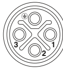
Pin assignment of M12 socket, 4-pos., S-coded, view of socket side
