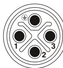
Pin assignment of M12 plug, 4-pos., S-coded, view of plug side
