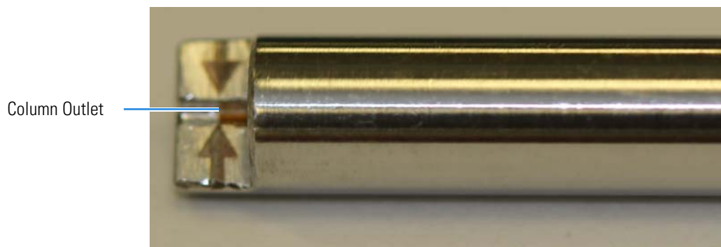
Figure 28. Lining Up the Column in the Column Measuring Tool
