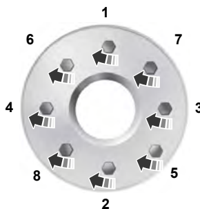
8-lug nut torque sequence
