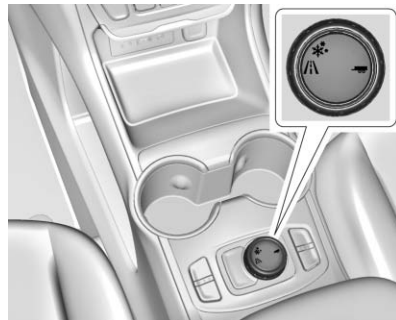
Driver Mode Control Knob for FWD
