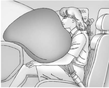
The front outboard passenger frontal airbag is in the passenger side instrument panel.
