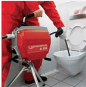
Manual feed is done by means of a working loop bend
