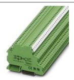
Input solid-state relay terminal block, input: 24 V DC, output: 3 - 48 V DC/100 mA, terminal block width: 6.2 mm
