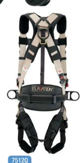
Elavation<sup>™</sup> Premium Harness with quick connect buckle chest connection, quick connect buckle leg connection, back and waist D-rings with backpad and toolbelt, 400 lb. capacity
