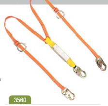
Tie-Back 6 ft., Dual Leg Energy Absorbing Lanyard, orange polyester web, with (3) snap hooks, 310 lb. capacity, 3,600 lb. rated hardware. Meets requirements of ANSI Z359.13-2009.
