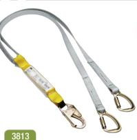
Tie-Back 6 ft., Dual Leg, Energy Absorbing Lanyard, gray polyester web, with (1) snap hook & (2) tie-back hooks, 310 lb. capacity, 3,600 lb. rated hardware. The thread will turn red when the product is worn out and needs replacing. Meets requirements of ANSI Z359.13-2009.
